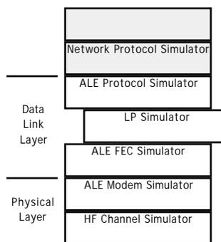
Figure 4: Simulator Stack
